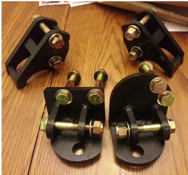
Figure 2: Lifted Brackets (Passenger side bracket on left, Driver side bracket on right)
