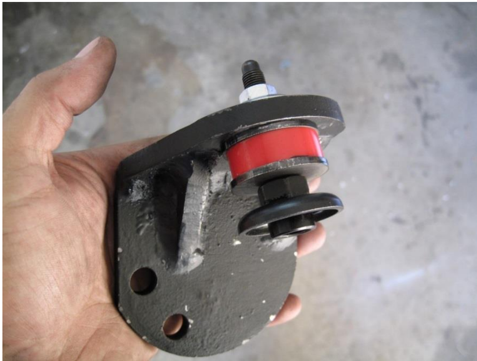
Figure 4: Stud Bushing on the Driver Side Bracket
