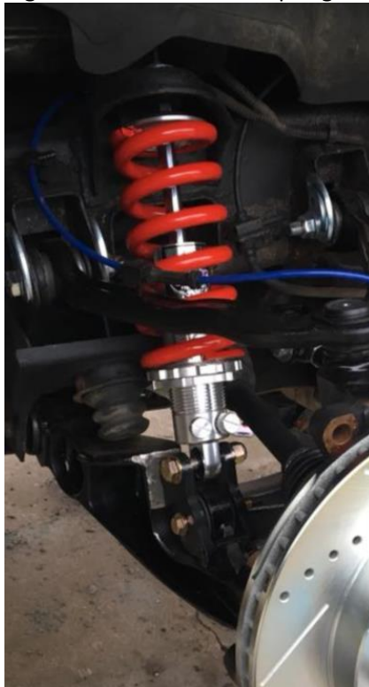
Figure 1: Full Normal Coilover Assembly
