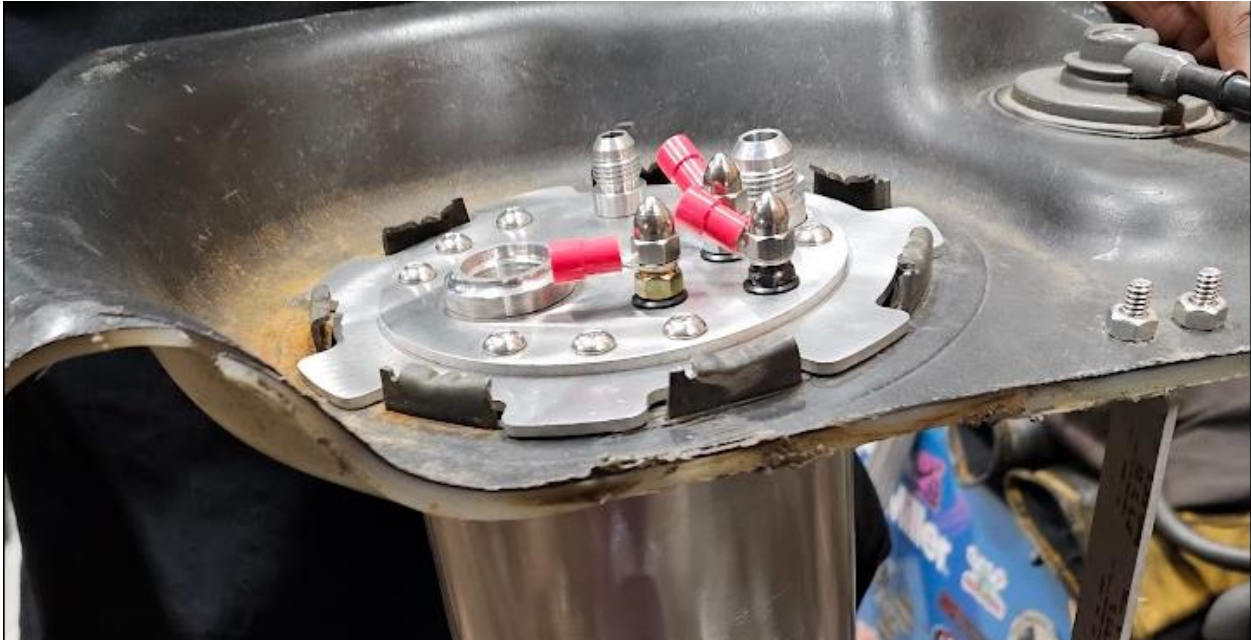
Figure 3: Surge Tank and Level Sensor Installed
